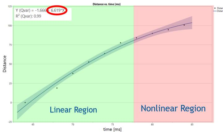
Figure 3: An example of the distance vs. time graph for PFV analysis discriminating between near field (linear region) and far field (non-linear region) regions from the mouthpiece edge.
