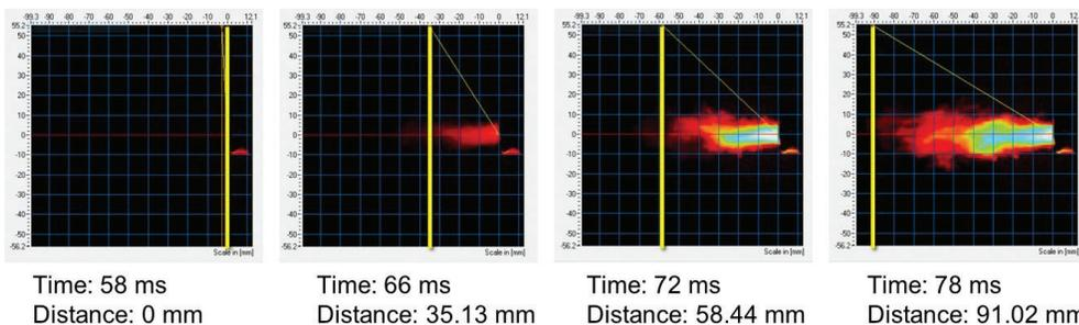
Figure 1: Time sequence of images of the emitted aerosol from a sideward view
