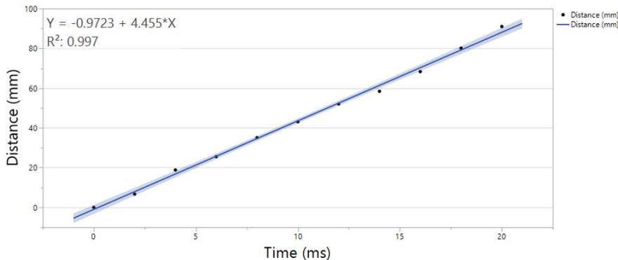
Figure 2: Relative distance vs. time graph of the leading edge plume. Velocity is calculated from the slope of the linear fit.
