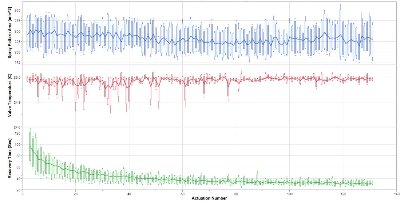
**Figure 1.** Boxplots of through-life baseline performance measured from four (4) product samples under isothermal valve conditions. Notice the dramatic drop in Recovery Time starting at about 2 minutes initially to about 30 seconds at the end of life. Through-life spray pattern area performance had a mean of 232.8 mm<sup>2</sup> with a S.D. of 31.2 mm<sup>2</sup>.
